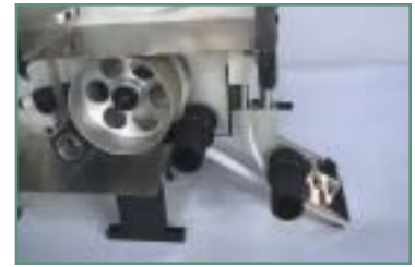
BK730 simple height adjustment and thread path
