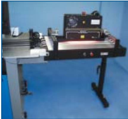
BK701 Vacuum Table Extension 3ft (option). Shown here with Research dryer #4540. (Dryer not included.)
